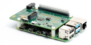
Shown assembled with RPi (not supplied) for full AST system demonstration.
