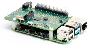
Shown assembled with Raspberry Pi (not supplied) for full AVS client demonstration.
